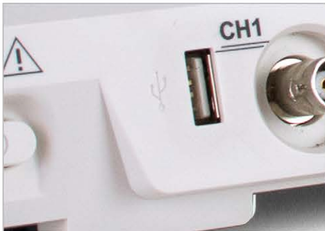
Front USB port, support U disk storage.
